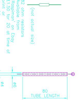
Available from most model shops. £2.50 for 1.0m at time of print Outside X Ø4 Inside. Aluminium Tube – ø6mm
